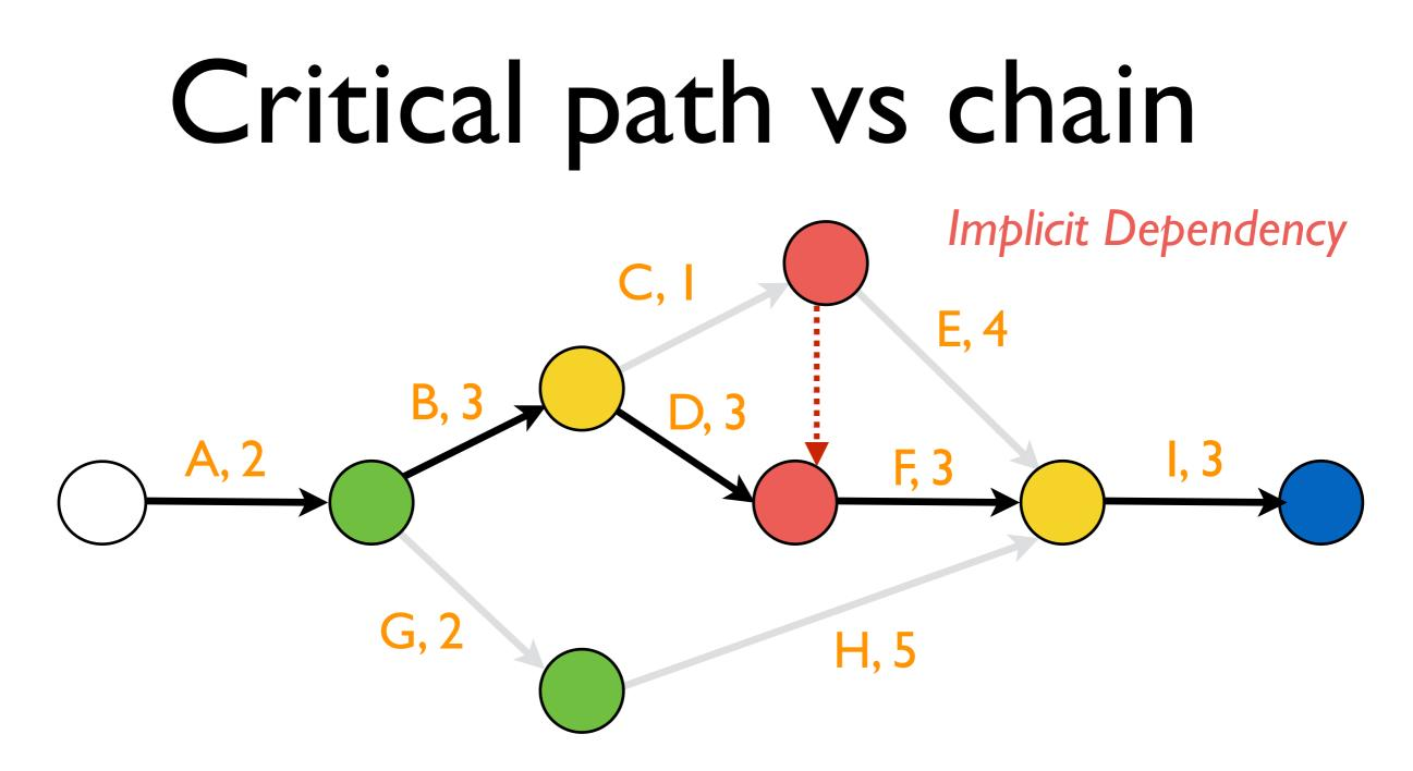
Critical path: A-B-D-F-I Critical chain: A-B-C-D-F-I When is critical chain the same as critical path?
