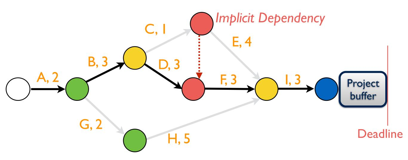
Feeding chain: path of activities merging into critical chain Feeding buffer: placed at the merge point
