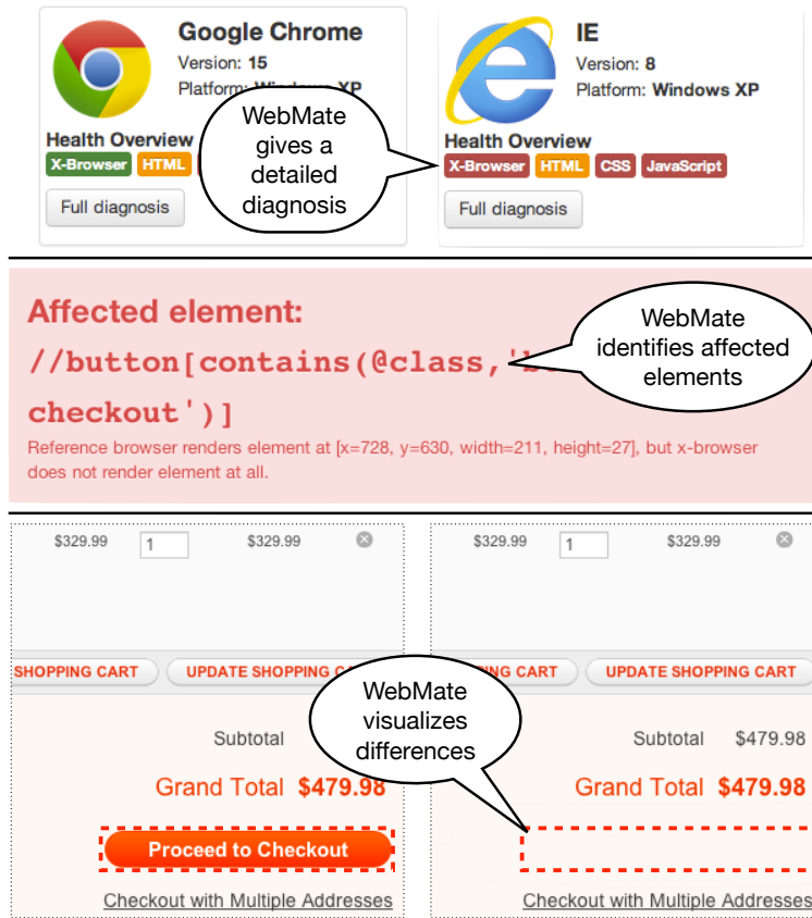
Fig. 2. Example of a diagnosis produced by WEBMATE. In Internet Explorer 8, the checkout button is missing. WEBMATE identifies the missing element and visualizes the problem using screen shots.
