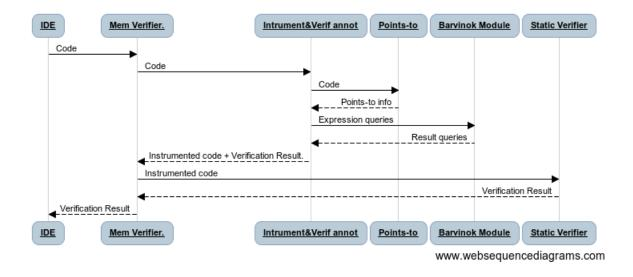
Figure 12: Interaction between main modules.
