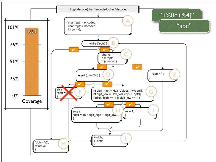
With another test case, we can cover this remaining branch – and find the defect.
