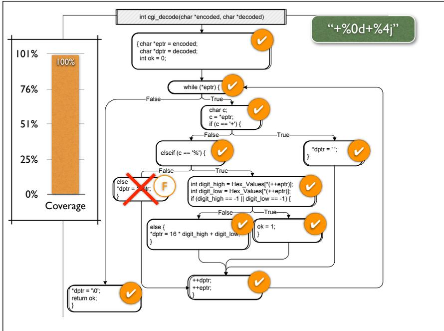
Why is branch testing useful? Assume block F were missing (= a defect). Then, we could achieve 100% statement coverage without ever triggering the defect.
