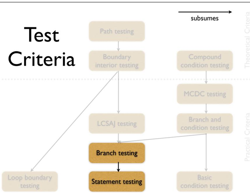
As an example, consider branch testing, which is a criterion that subsumes statement testing. In other words, if the branch testing criterion is satisfied by a pair  $\langle \text{program}, \text{test suite} \rangle$ , so is the statement testing criterion for the same pair.
