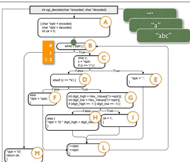
With these three test cases, we obtain loop boundary adequacy for the cgi\_decode main loop.
