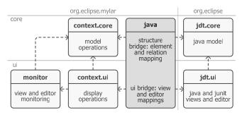
Figure 2: Mylar plug-in architecture and Java bridge
