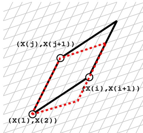
The transformation that transforms the black figure into the red figure (called *shearing*) is *area-preserving*.
