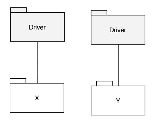
... but we must construct drivers for each module (as in unit testing) ...
