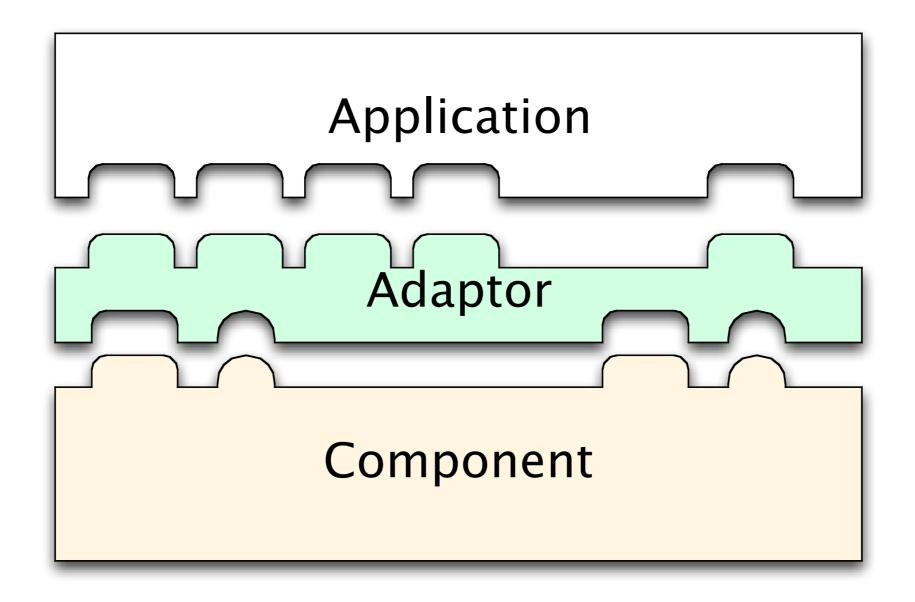
Applications often access components through an adaptor, which can also be used by a test driver
