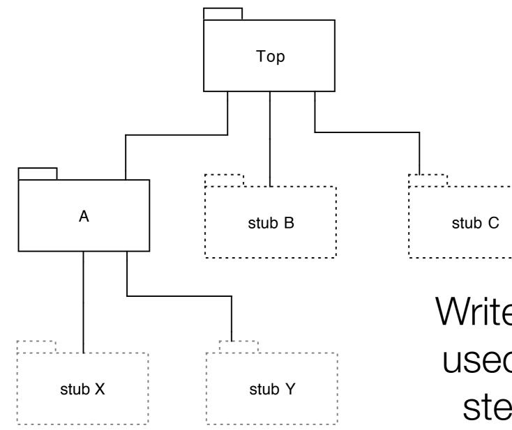
Write stubs of called or used modules at each step in construction
