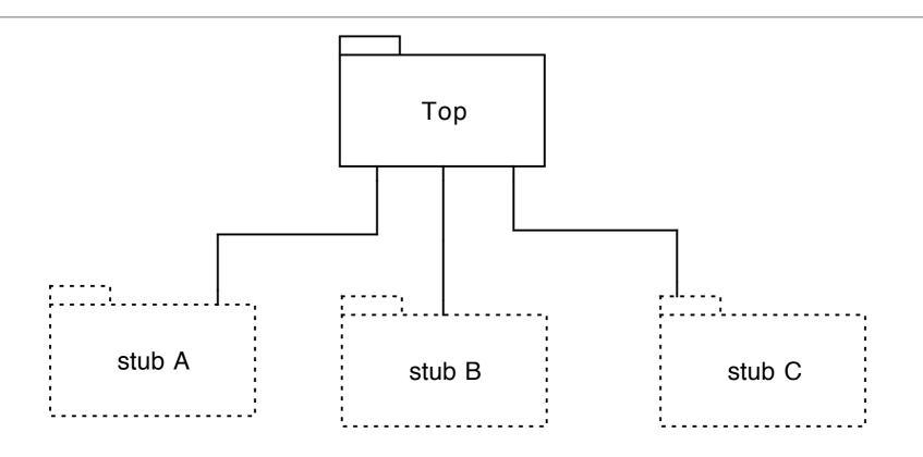
Working from the top level (in terms of "use" or "include" relation) toward the bottom. No drivers required if program tested from toplevel interface (e.g. GUI, CLI, web app, etc.)
