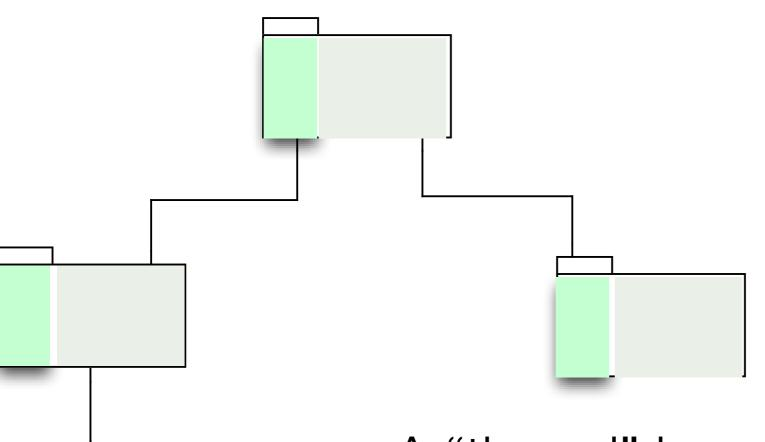
A "thread" is a portion of several modules that together provide a user-visible program feature.
